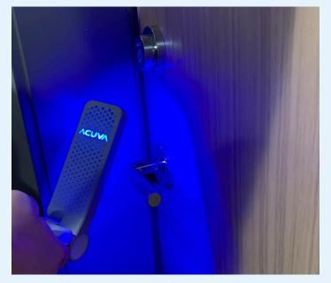
Blue LEDs to show visible mapping of disinfection area
