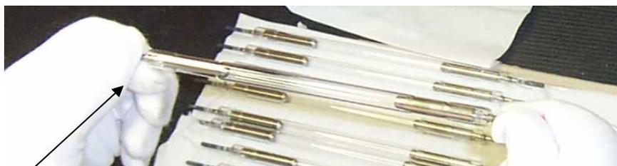
Lamp being well supported at both ends
