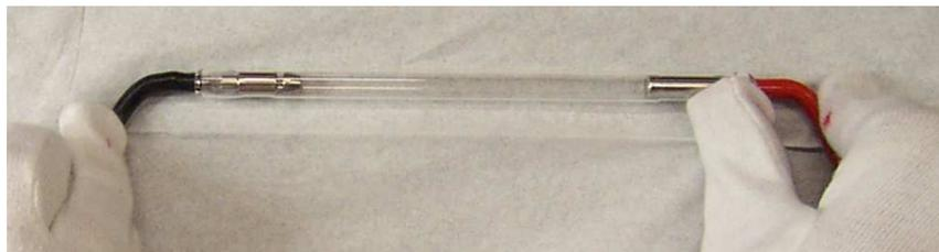
Lead wires being bent and the lamp being support
